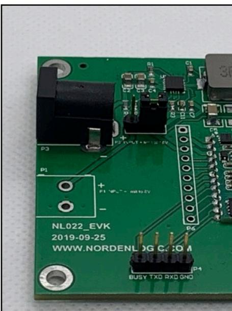
The NL022\_EVK board is by default configured to be used with 58mm print heads (see support print head types at the beginning of this document). In order to configure the EVK board for supported 80mm print head types the jumper P8 and P9 must be configured.
